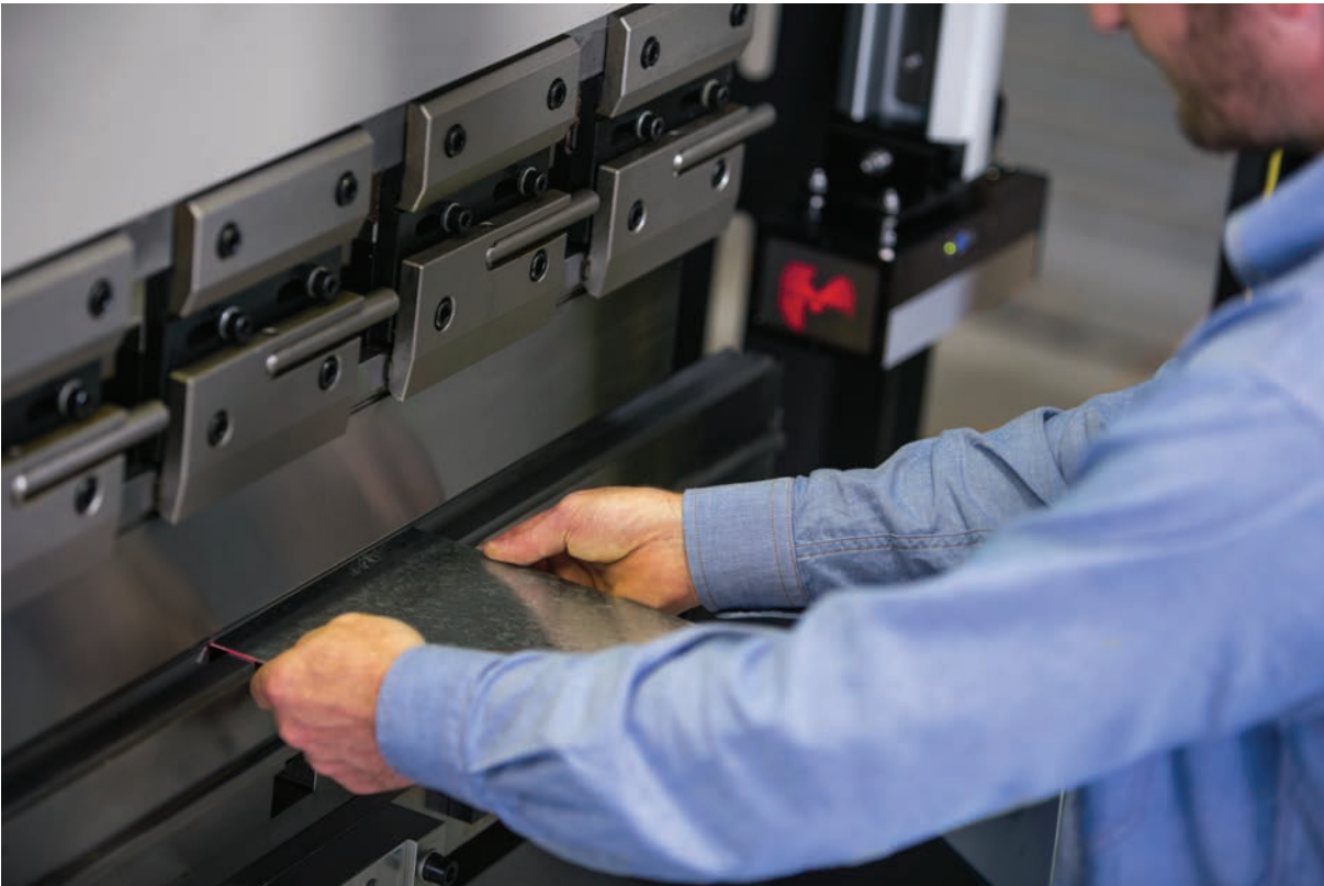
Close proximity protection enables safe handling of the work piece during high speed closing.
